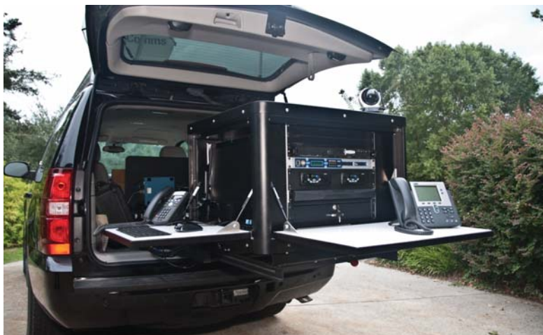
Shown mounted on slide-out rails, the system can be mounted in a conventional electronics rack or wherever required.
